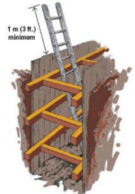
*This is an example of ladder use in an excavation over 1.2 m (4 ft.) deep.*
